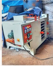
Compact yet efficient, our 6, 8, 10 tray dryers delivers precision drying with a batch capacity of 25, 40 & 50 kg. Ideal for small-scale operations.
